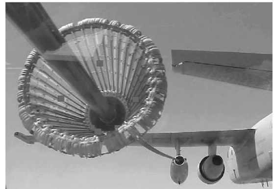
Fig. 4 Candidate beacon configuration for AAR, as seen from VisNav sensor.
